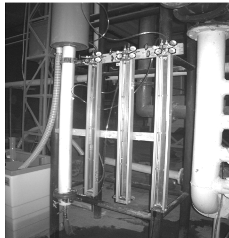
Photo 2. General view of the equipment with indirect manometers
