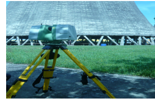
Fig.3 C10 ScanStation scanning system
