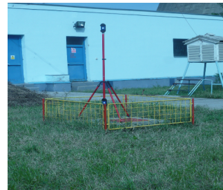
Fig.4 Scanning prism pole with tripod mounting
