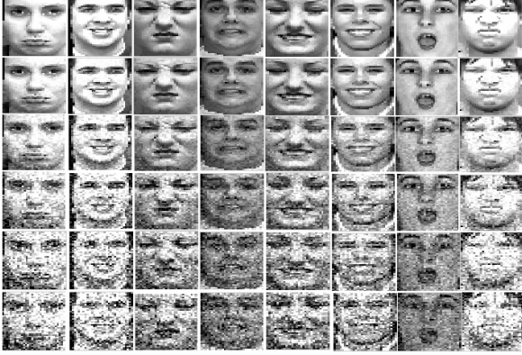
Figure 1 Each row depicts eight samples from the C-K test set for different noise levels expressed through SNR. First row illustrates noise-free face images, following, from top to bottom, images having different SNR values varying as \text{SNR} = \{20, 10, 5, 2, \text{and } 1\} .
