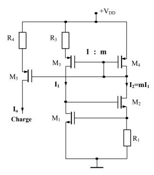
Fig.3. Final reference-current source with output towards the charge with grounded end
