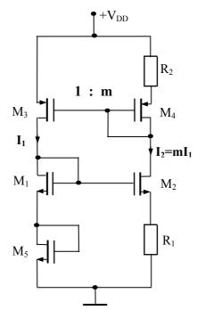
Fig.1. Second-order temperature-compensation branch-current reference (Fiori-Crovetti)
