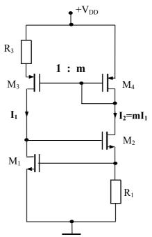
Fig.2. Proposed second-order temperature-compensation branch-current reference
