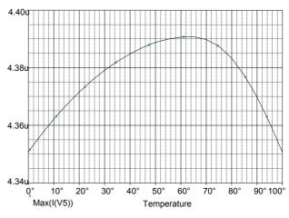
Fig.4. Reference-current variation against the temperature
