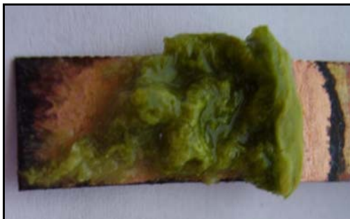
Figure 4. Macroscopic aspect of electrodeposition for samples 3 (1 mV/s)
