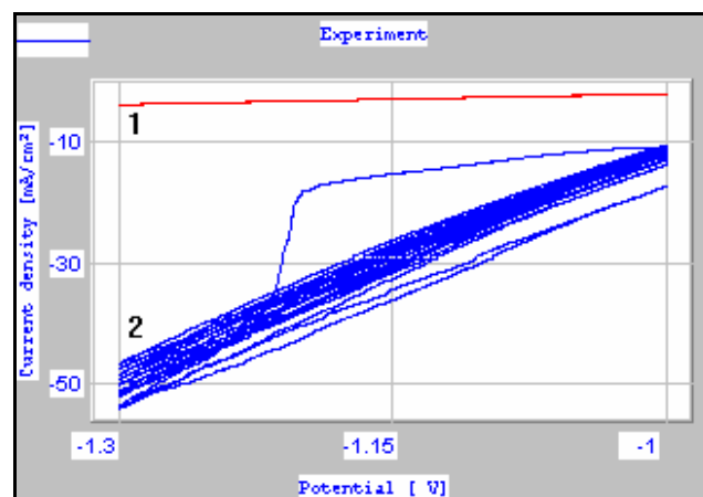
Figure 2. Voltammograms for sample 2, at potential (-1000)-(-1300) mV, scan rate = 10 mV/s 1 – electrolyte support HCl 2N; 2 – sample 2
