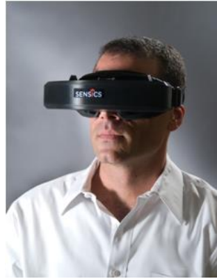
Figure 2-3 Head worn device for augmented reality (image from Sensics Inc. via Wikipedia licensed as CC BY-SA 3.0 [31])
