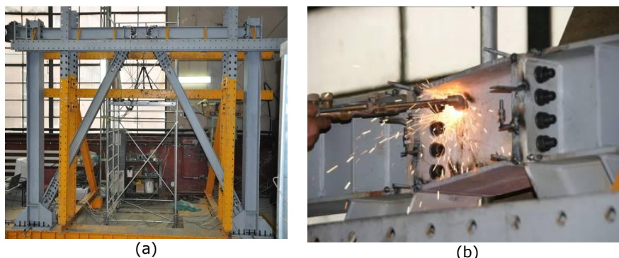
Fig. 3-24. One storey frame: (a) experimental setup and (b) flame cutting of the link.
