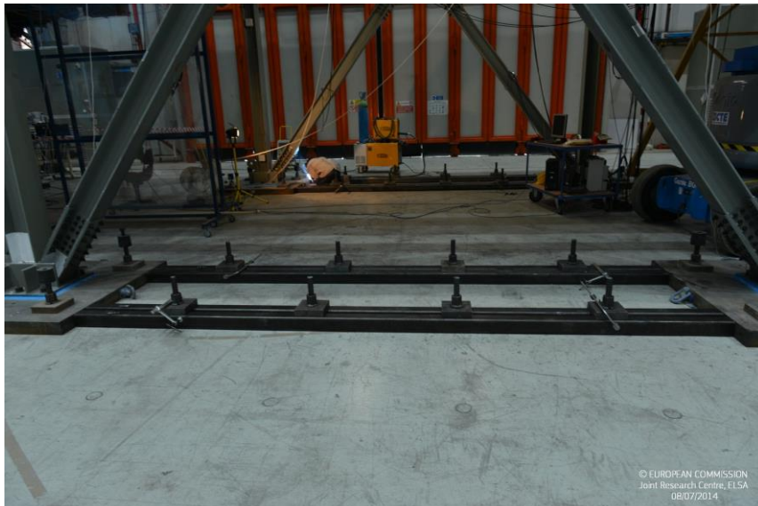
Fig. 4-55. Additional fixing of the columns
