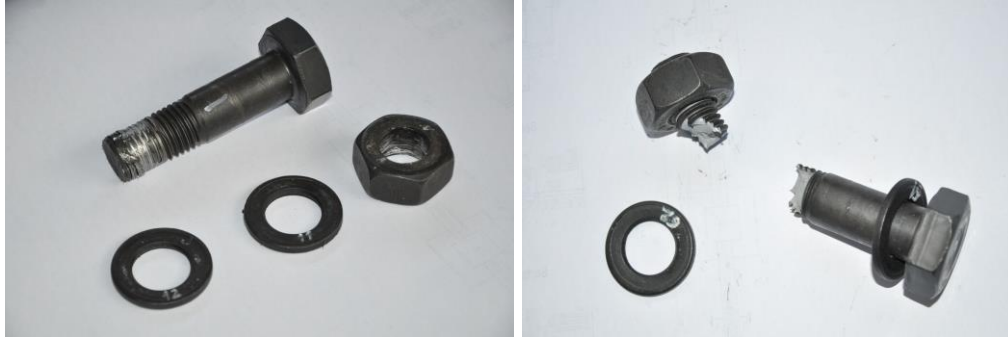
Fig. 4-8. Bolt failure modes
