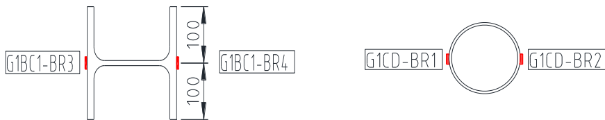
Fig. 4-33. Strain gauges position on EBF braces and an damper braces
