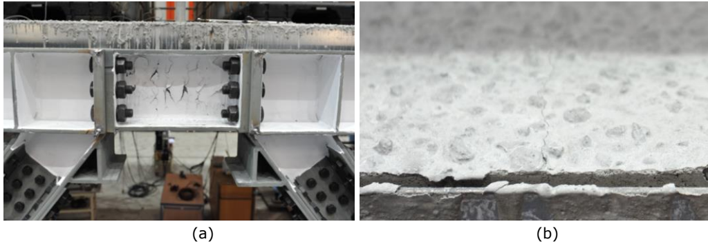
Fig. 4-37. Link behaviour (a) and concrete slab state (c) at the end of DL test
