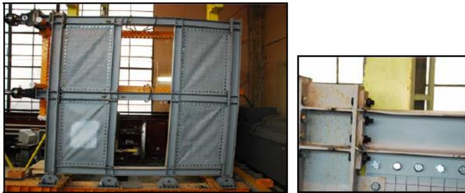
Fig. 2-34. Tested specimen and connection detail [62]
