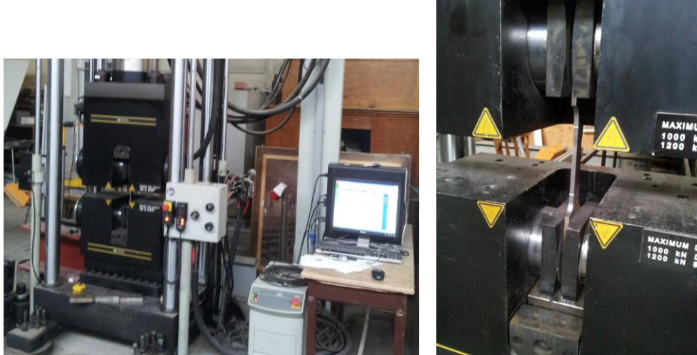
Fig. 4-2. Tensile test on steel sample
