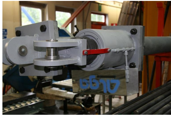
Fig. 4-17. Braces with dampers
