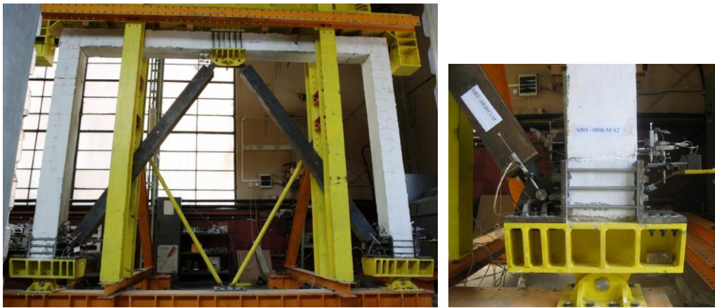
Fig. 2-29. Experimental tested frame view and connection detail [49]
