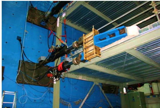
Fig. 4-20. First storey actuators
