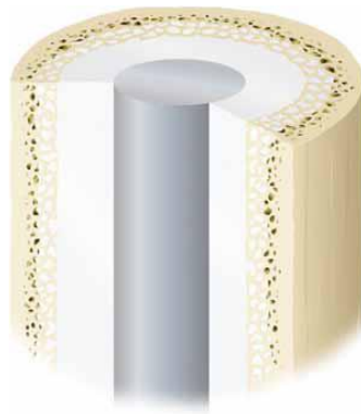
Figure 22. Section view representing a cemented stem and cement penetration
