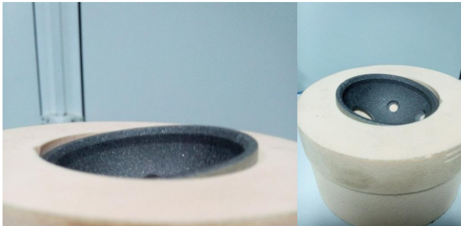
Figure 90. Representation of cup failure (3 mm offset)
