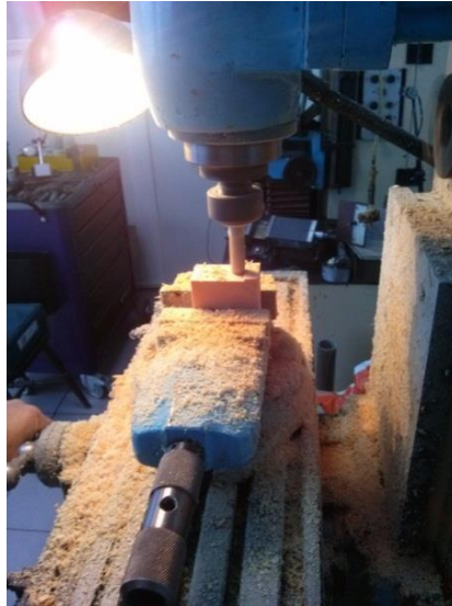
Figure 75. Foam block preparation using a milling machine
