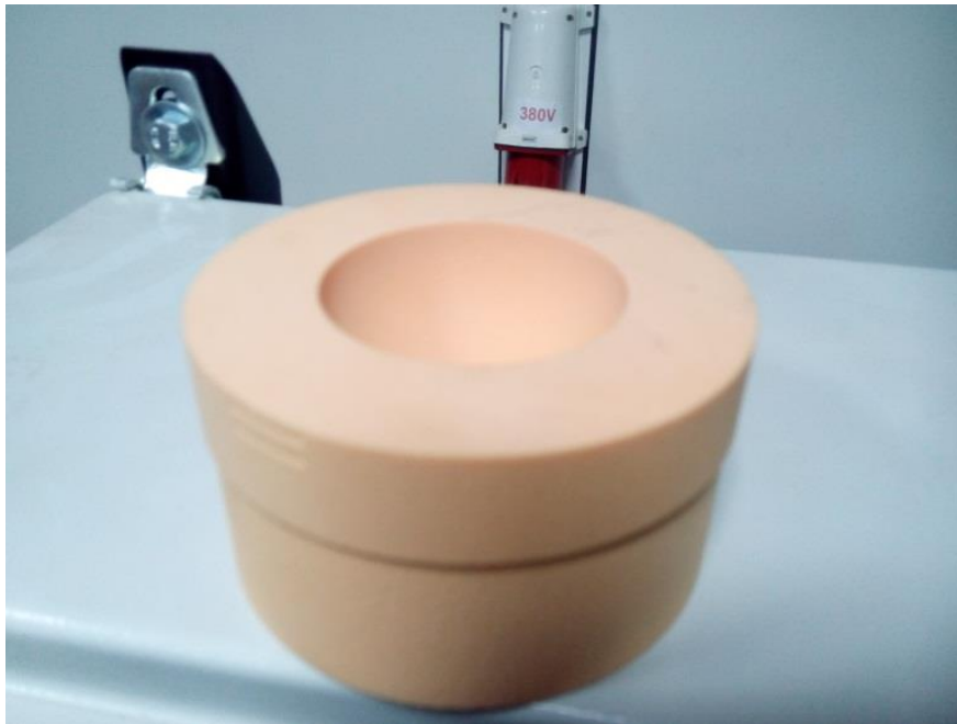
Figure 87. Test block specimen with prepared acetabular cavity
