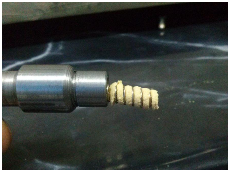
Figure 84. Mode of failure for the medical screws
