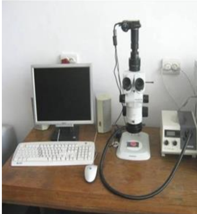
Fig. 2.10 Steromicroscopul optic OPLIMPUS SYX7 (foto: Lavinia Mădălina Micu)
