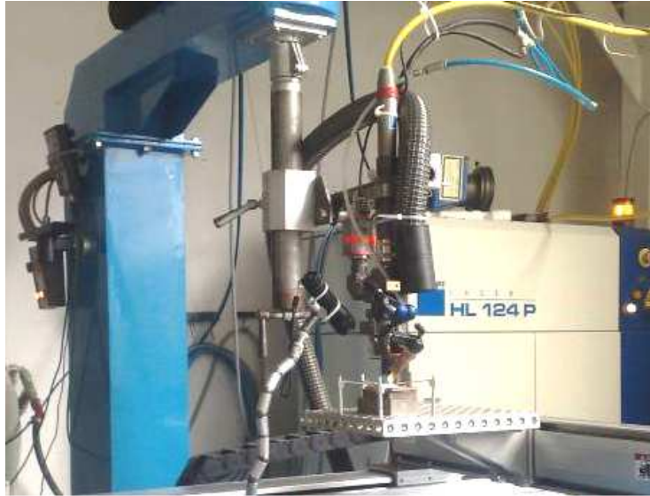
Fig.5.14 Standul Trumph HL 124 P LCU dotat cu laser pulsat programabil Nd-YAG (foto de la ISIM - Timișoara)
