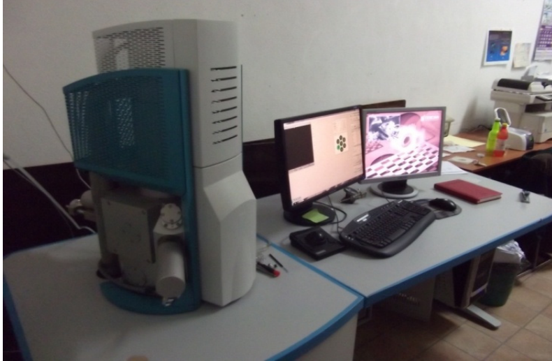
Fig. 2.11 Microscopul electronic cu baleiaj TESCAN VEGA 3 LMU Bruker EDX Quantax
