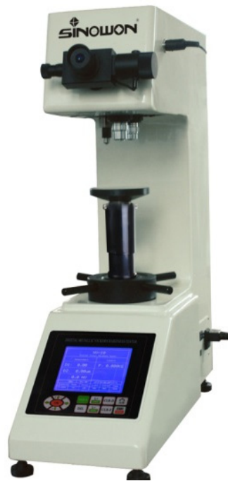
Fig. 2.16 Durimetru digital Vickers model HV-50AC.
