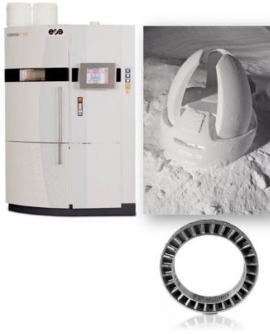
Figure 2.25. Exemplary – SLS machine and SLS and SLM products. [15] [Fraunhofer IPA]
