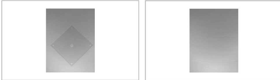
Figure 6.12. Undistorted area: I4QC in IM1 (left a sintered layer and right a powder layer).
