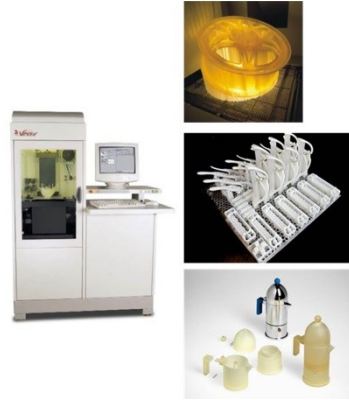
Figure 2.12. Exemplary - SLA machine and products. [9]
