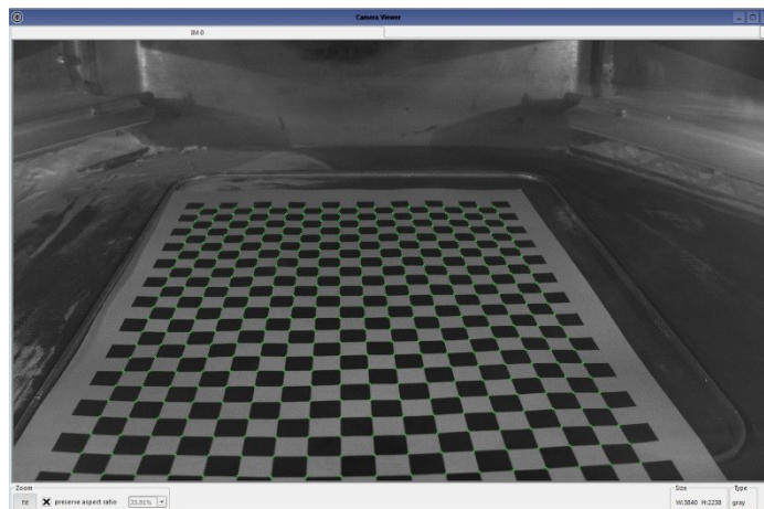
Figure 6.11. Square corners in chessboard, used for a part of the building platform, where the objects are manufactured.
