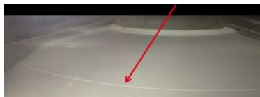
Figure 4.6. View of the powder layer after application - serious defect in the powder layer. [source: Fraunhofer IPA: EOS FORMIGA P 100]
