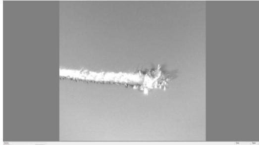
Figure 6.17. Exemplary: powder layer with serious, wide failure.
