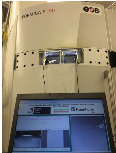
Figure 7.3. Hardware and software integration in final system: implemented level.
