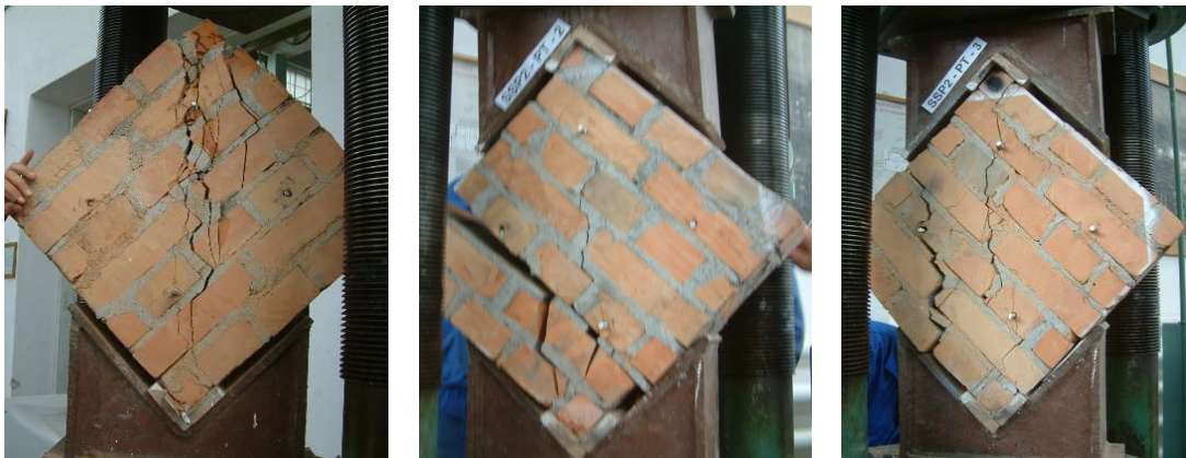
Connection realized with prestressed ties
