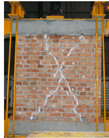
Figure 4-34. Experimental behaviour curves and failure mode for cyclic specimens
