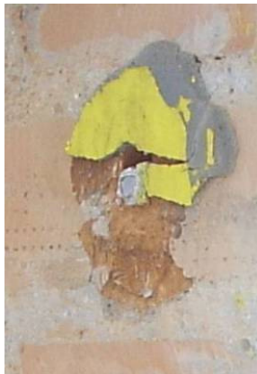
Figure 4-11. Failure modes for chemical anchor connections
