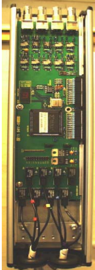
Fig. 7.3 Physical layout of the Interface and Protection Card for the power inverters
