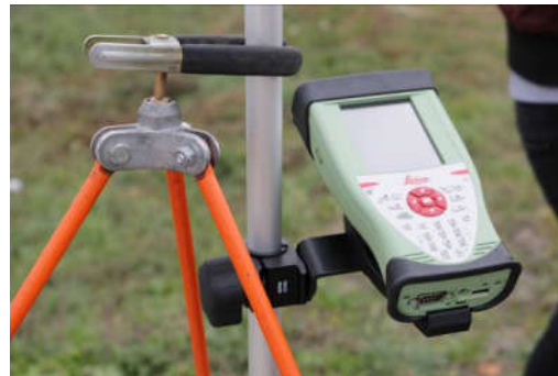
Fig. 2.7 Receptor GNSS, modelul Leica GS08 (Șmuleac A., 2017)
