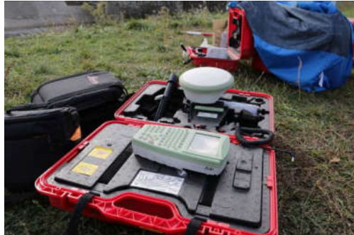
Fig. 2.6 Receptor GNSS, modelul Leica 1200 (Șmuleac A., 2017)
