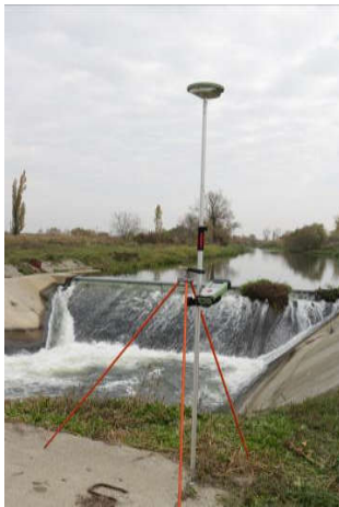
Fig. 2.6 Receptor GNSS, modelul Leica 1200 (Șmuleac A., 2017)
