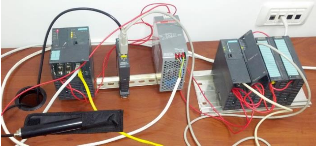
Fig. 5.19. Experimental setup – main parts (in order from left to right): antenna, teleinterface module, GPRS modem, power supply, PLC with teleinterface module
