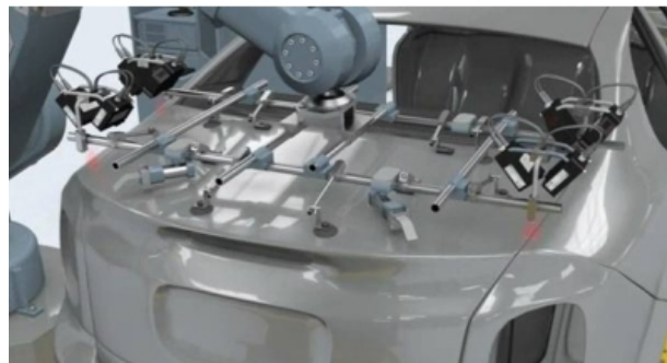
Figure 2.21: An illustration of the VMT-BestFit system mounting a trunk lid.
