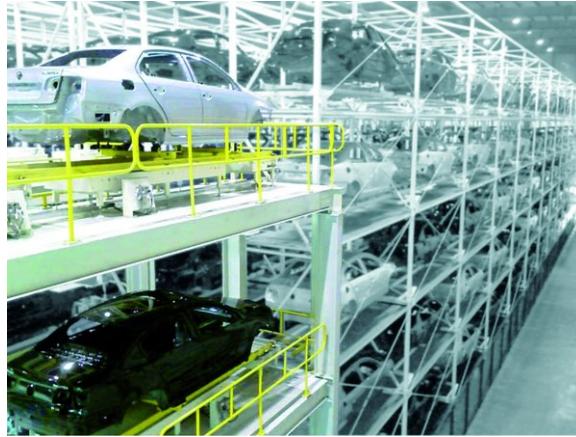
Figure 1.4: A high rack storing multiple painted car bodies.
