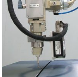
Figure 2.19: Robot wrist with sensor at roof-ditch application
