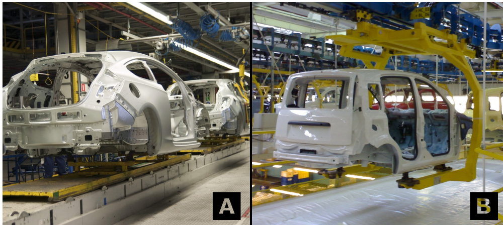
Figure 1.6: Image A: Car bodies on a skid conveyor. Image B: Painted body on an overhead conveyor
