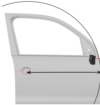
Figure 5.1: Measurement positions at a door with the corresponding osculating circle.
