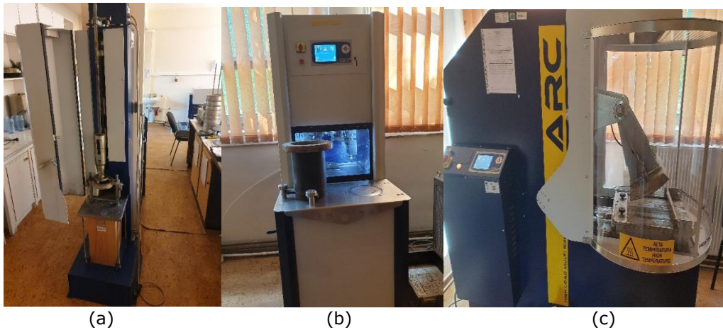
Figure 3.6. (a) Matest Marshall impact compactor; (b) Matest gyratory compactor; (c) Roller compactor - Road Laboratory, University Politehnica Timisoara.
