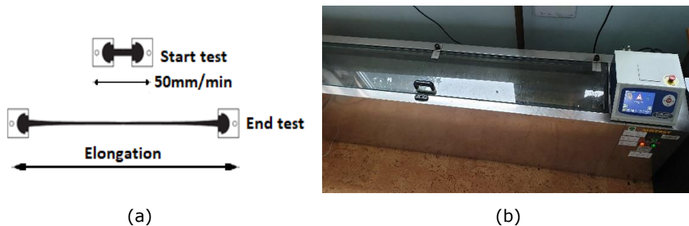
Figure 2.6. (a) Elongation test principle; (b) Ductilimeter Matest® - Road Laboratory, University Politehnica Timisoara.
