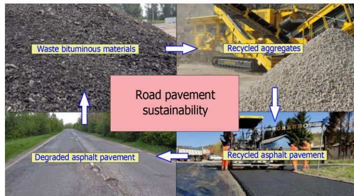
Figure 1.25. Road pavement sustainability – recycling/reusing of waste asphalt materials.
