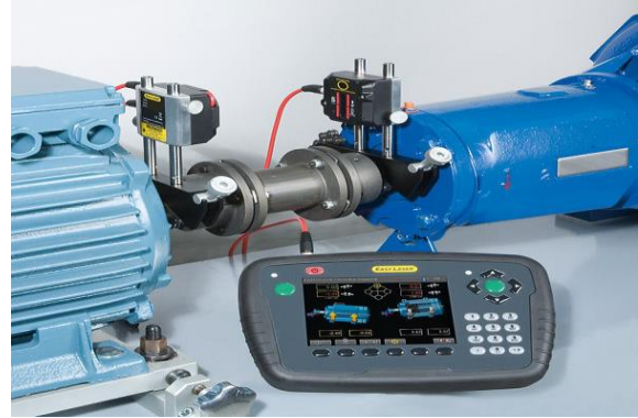
Figure 7. Laser shaft alignment method using EasyLaser system Damailini [5]
