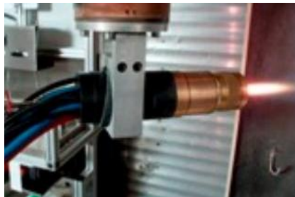
Figure 1.9 Axial III plasma spray torch (courtesy of Mettech Corporation)
