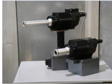
Figure 1.17 M2 AC-HVAF gun (courtesy of Uniquecoat)
