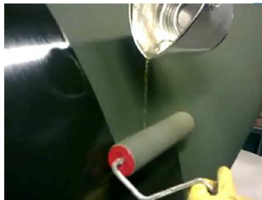
Figure 1.29 Application of sealers on thermally sprayed coating
