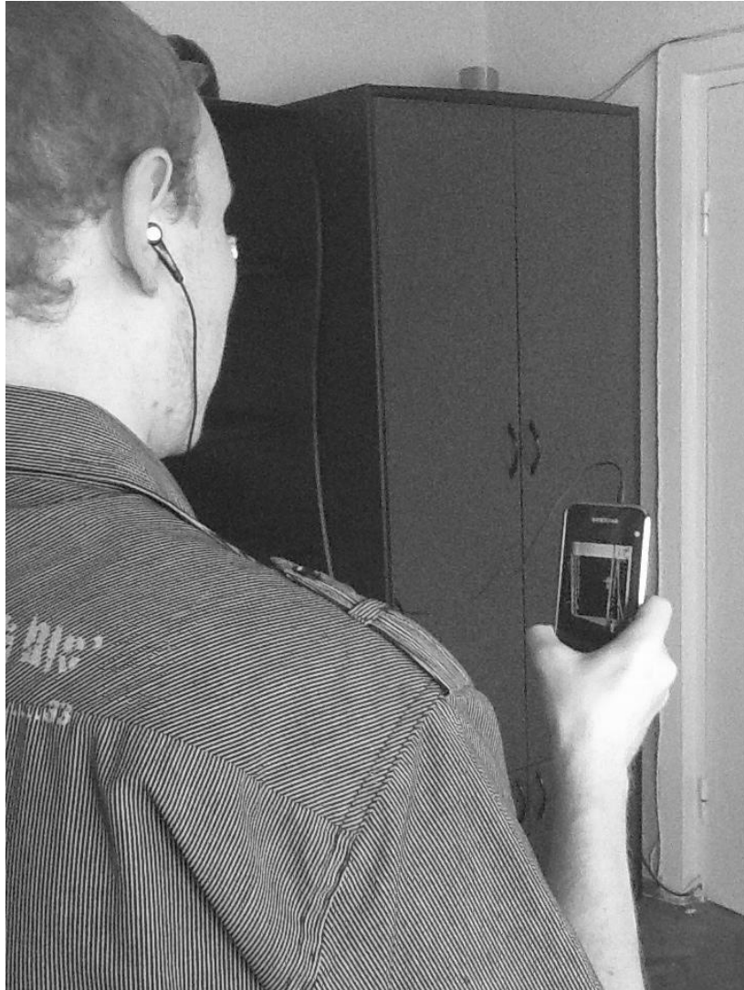
Fig. 4.49 Indoor usage of the obstacle detection implemented as an application for a smartphone (obstacle in this case is a closed door). When the person is approaching the closed door a beep is send to the headphones signaling the obstacle.
