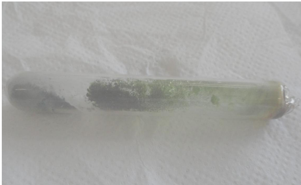
Figure 5.1.1. Photo graph of the vacuum sealed quartz tube after the thermal treatment
