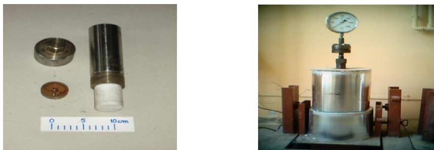
Figure 3.1. Teflon liners and steel covers used as autoclaves (a) subcritical, and (b). supercritical conditions
