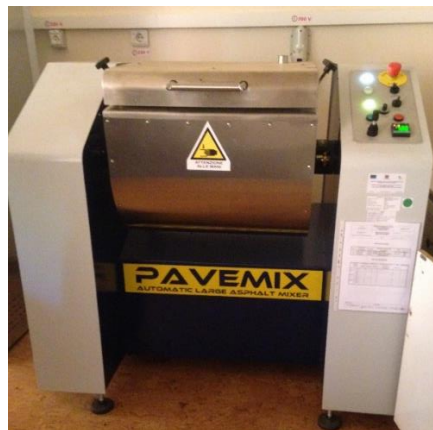
Figura 3.6 – Malaxor mecanic de laborator
