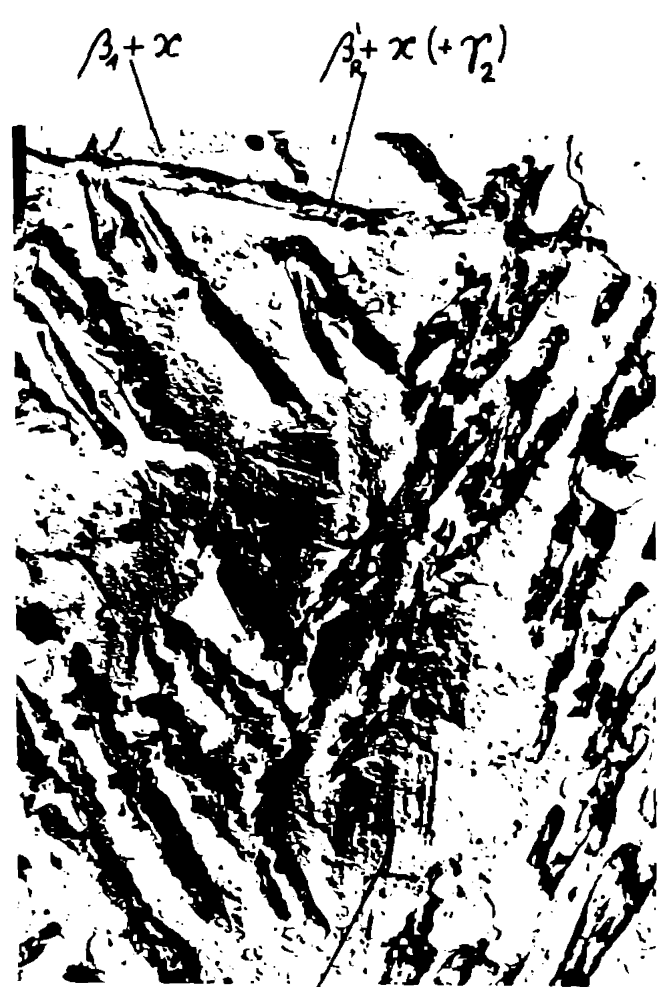
Fig.6.10. Turnat+călire 950°C+ revenire 500°C/30 min/H 2 O (atac electrolitic) M.E.T.x4700
