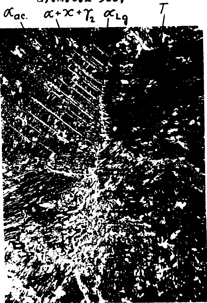
Fig.6.15. Furnat + cãlire 1000°C + revenire 450°C/45 min/aer
