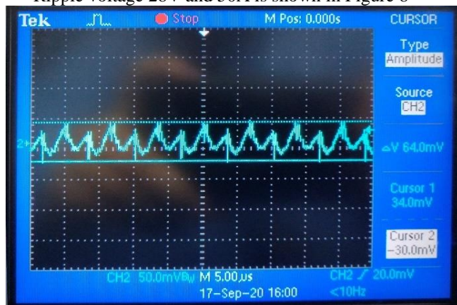
Figure 8: Ripple voltage at Vin-nom and Iout-max
