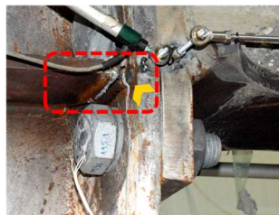
Fig. 3-37. Monotonic response: a) M-\phi curve (bending moment, rotation at column centreline); b) specimen in maximum hogging "1"; c) significant cracks in the concrete slab "1"; d) stiffener weld failure "2"; e) lower beam flange-to-end-plate weld failure "3"
