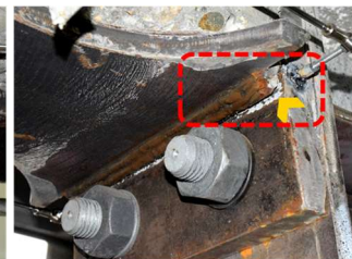
Fig. 3-37. Monotonic response: a) M-\phi curve (bending moment, rotation at column centreline); b) specimen in maximum hogging "1"; c) significant cracks in the concrete slab "1"; d) stiffener weld failure "2"; e) lower beam flange-to-end-plate weld failure "3"
