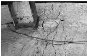
Fig. 3-37. Monotonic response: a) M-\phi curve (bending moment, rotation at column centreline); b) specimen in maximum hogging "1"; c) significant cracks in the concrete slab "1"; d) stiffener weld failure "2"; e) lower beam flange-to-end-plate weld failure "3"
