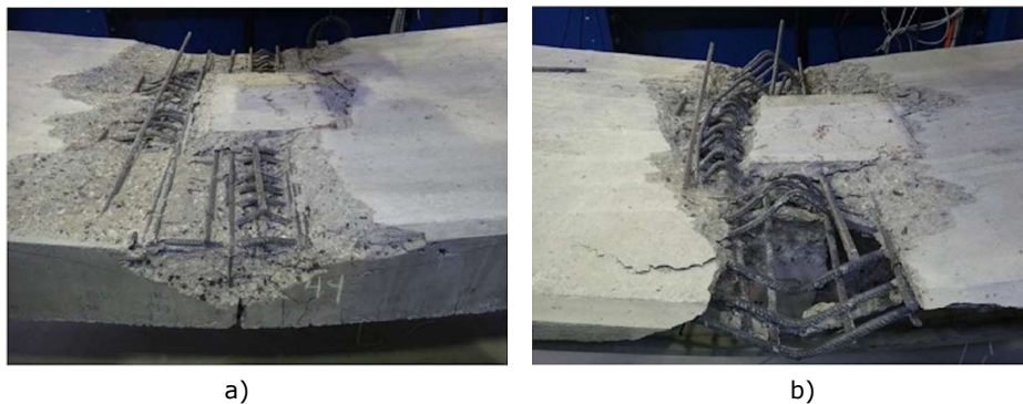
Fig. 2-20. Images from Kyriakopoulos et al. [44]: degradation state of specimens at the end of the tests: a) type 1 ; b) type 2
