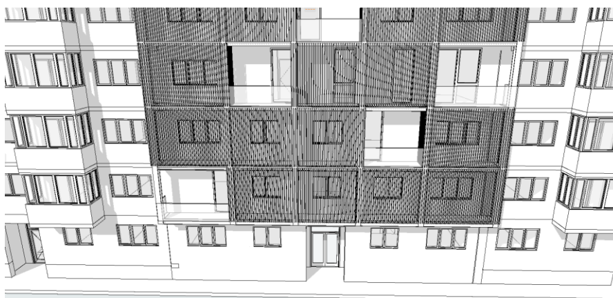
Figure 5.25. Concept image of the additional structure
