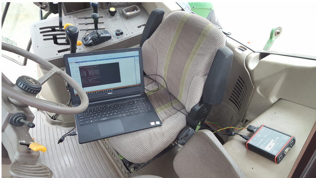
Figure 1.1: A typical heavy-duty vehicle implementing the SAE J1939 standard and tools for data collection of the SAE J1939 CAN traffic
