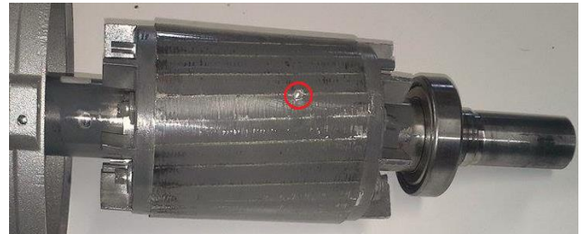
Fig. 6. Incipient outer cage bar fault
