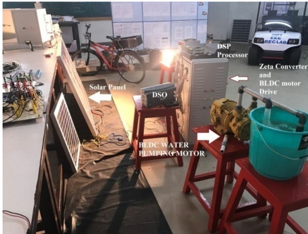
Fig.15. Experimental set up of proposed solar powered brushless dc motor based water pumping system
