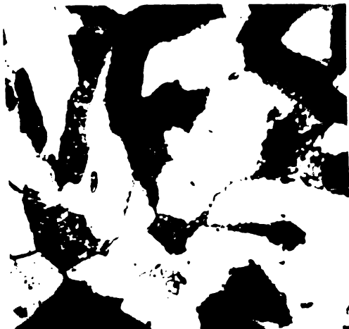
OLC 35 ×400 Deformare V_i = 58\% \Sigma = 58,5\% central
