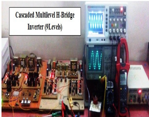
Fig.20. Experimental arrangement (b) CHBMLI (nine levels)
