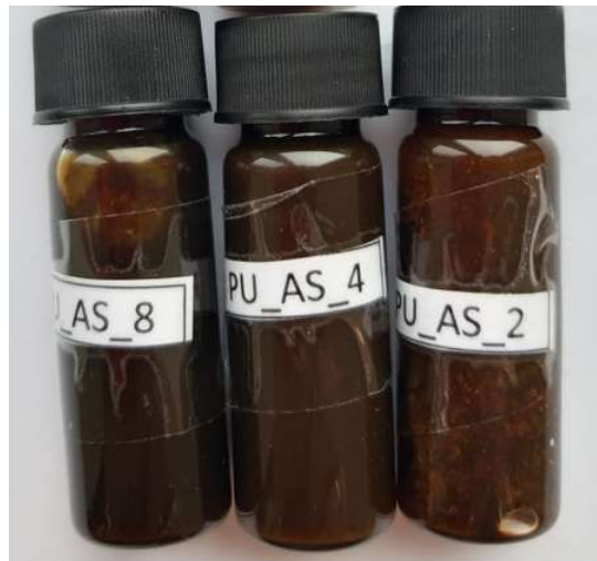
Figure 2.9 Acidolysis products obtained by acidolysis in autoclave with various carboxylic acids, as described in Table 2.10
