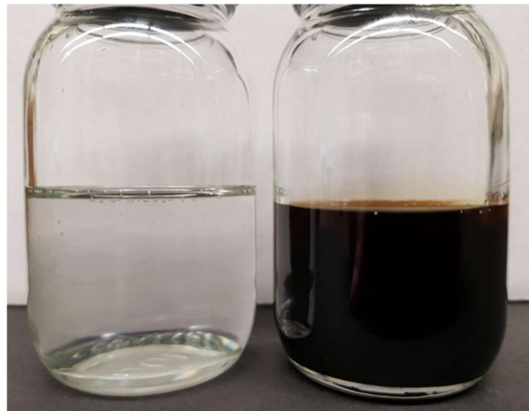
Figure 2.3 Glycolysis product obtained from flexible PU foam waste and diethylene glycol in a 1:1 (w/w) ratio, in autoclave (image on right), compared to virgin polyol (image on left)
