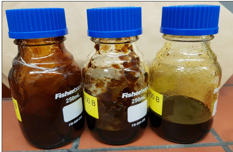
Figure 2.1 Glycolized products obtained using (a) atmospheric pressure method, (b) autoclave, and (c) microwave
