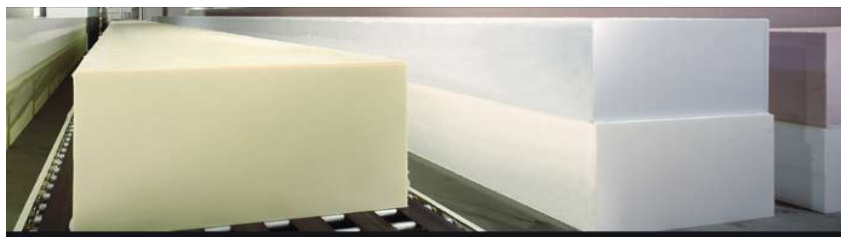
Figure 1.6 Polyurethane slabstock foam block, 60 m long, 2 m wide, and 1.2 m high [17]
