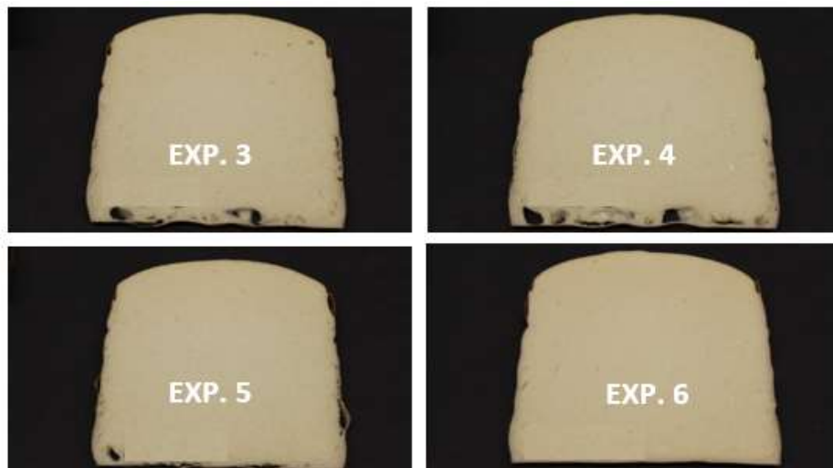
Figure 2.33 Vertical foam slice with different amine catalysts in the formulation presented in Table 2.16
