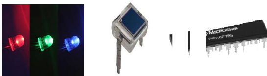
(RGB + NIR) leds BPW34 photodiode PIC16F785
