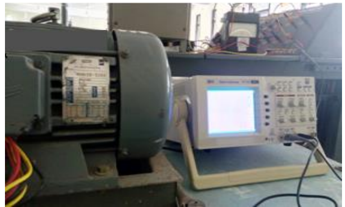
Figure.2 Experimental setup of three phase IM with shorting in one phase
