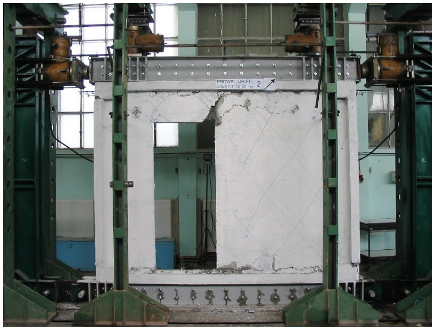
Figure E.18 Specimen PRCWP 3-S/E1-T at failure (0.7% drift ratio)
