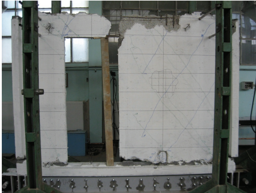
Figure E.33 Failure detail PRCWP 3-S/E1-T: general view after the crushed concrete was removed
