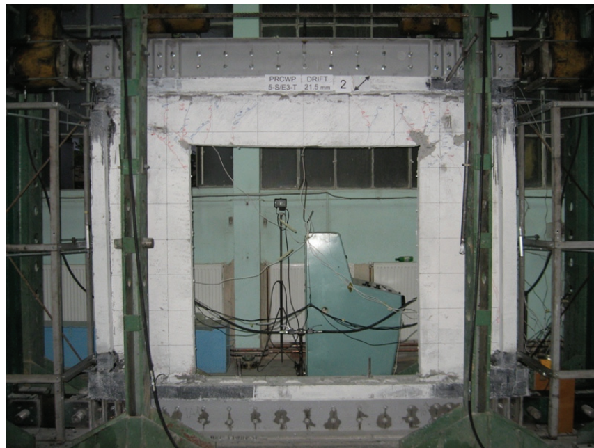
Figure E.34 Specimen PRCWP 5-S/E3-T at failure (1% drift ratio)
