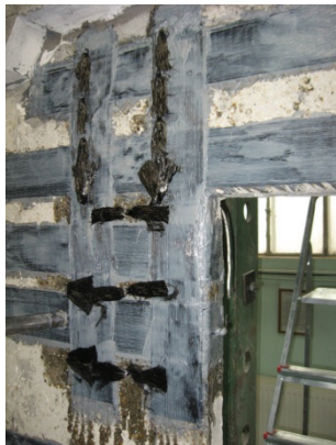
Figure B.5 FRP layout detail at the pier-to-beam connection of PRCWP 3-S/E1-T/R
