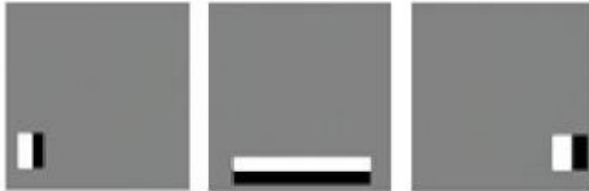
Figure 2. The used vehicle's features by Haar-Like filter
