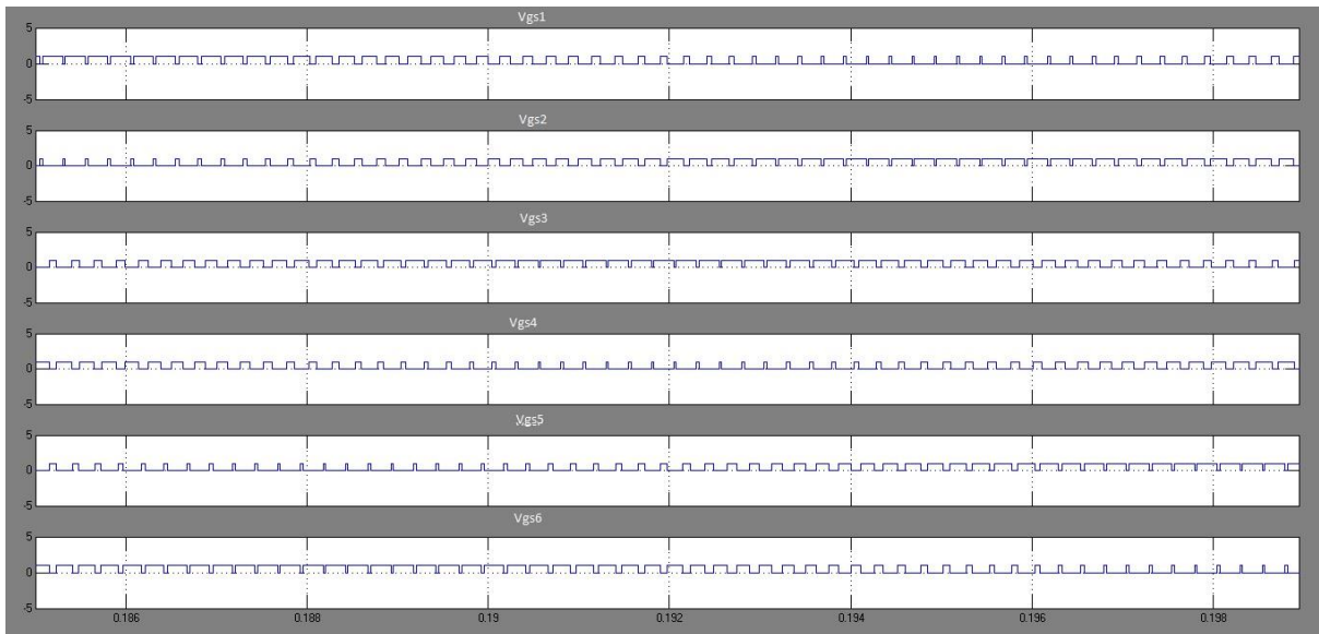
X-Axis: Time Y-Axis: Voltage Figure 12 Gate signals for SVPWM based BLDC motor drive
