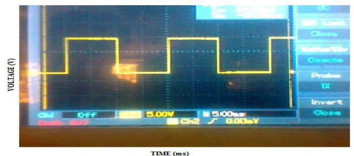
Fig.11 Control pulses from Control Circuit
