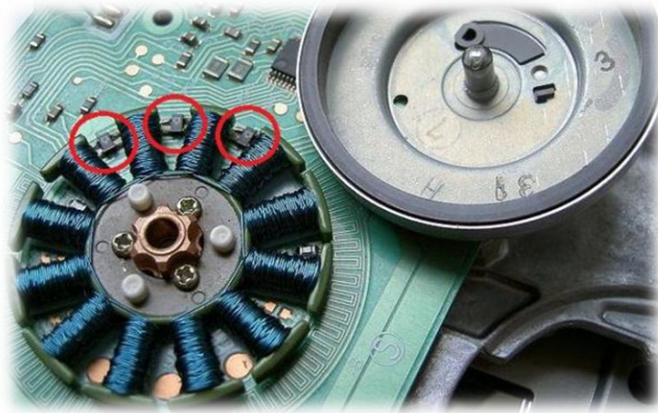
Fig. 1.19 Hall sensor placement of an outer rotor spindle floppy disk driver BLDC motor [17]
