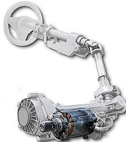
Fig. 3.7 Adaptive electronic steering system using BLDC motor [110]
