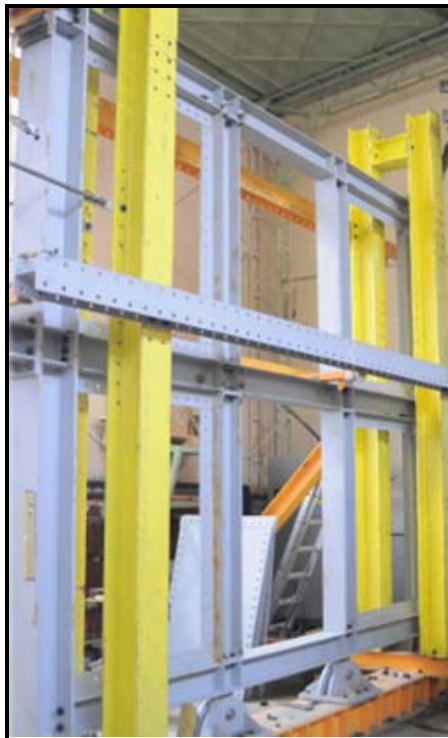
Figure 11 – Frame without infill plates
