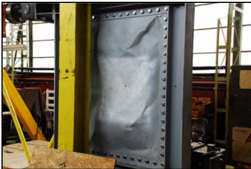
Figure 33 - Frontal view of infill plate
