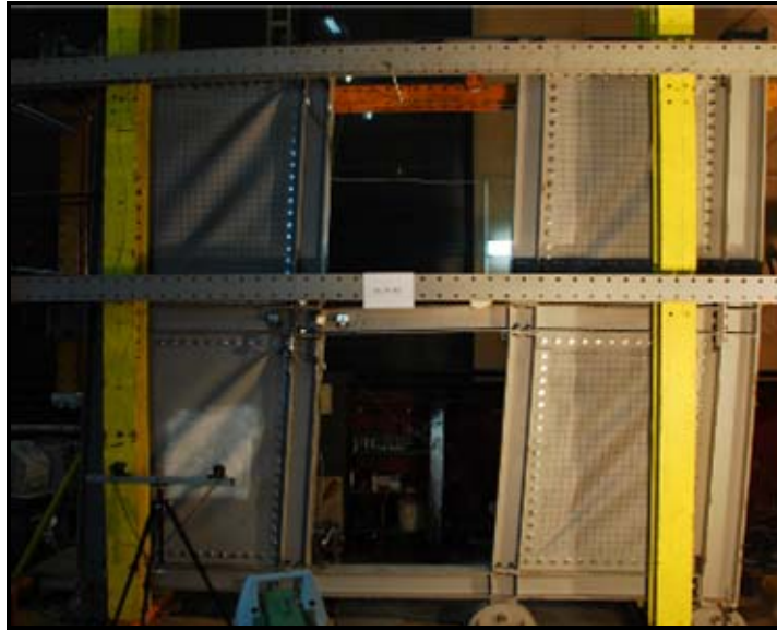
Figure 16 - Base shear force of 1150 kN (peak capacity)
