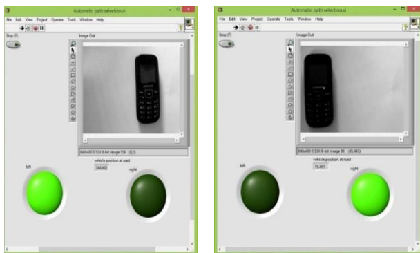
Fig 12. a). Left Obstacle Detection using NI Vision Assistant b). Right Obstacle Detection using NI Vision Assistant
