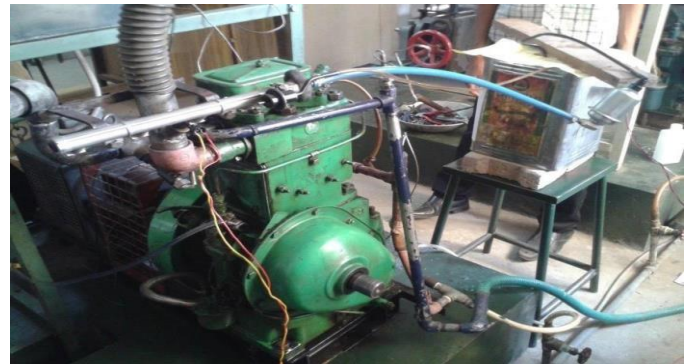
Fig 2. Engine Hardware setup for ethanol fumigation
