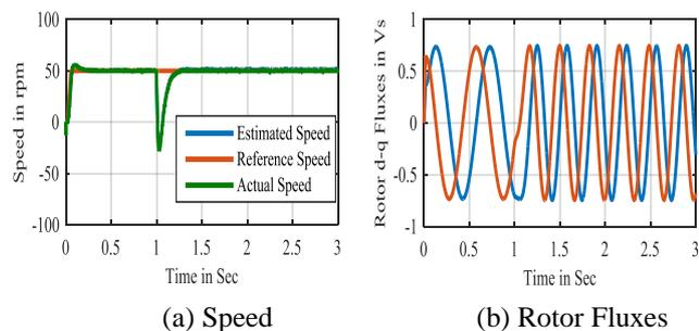
Fig.15. Performance under Test2 with Fuzzy controller
