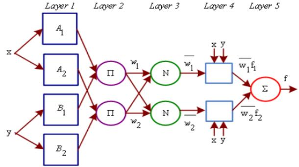
Fig.7. ANFIS structure with 2 inputs and 1 output
