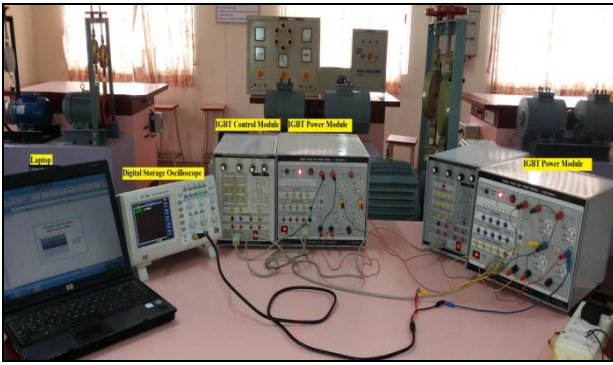
Fig. 13. Laboratory experimental arrangement
