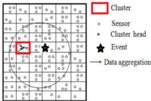
Fig. 1. Clustering and Data Aggregation
