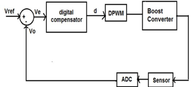
**Fig. 3.** Closed loop discrete controller for boost converter
