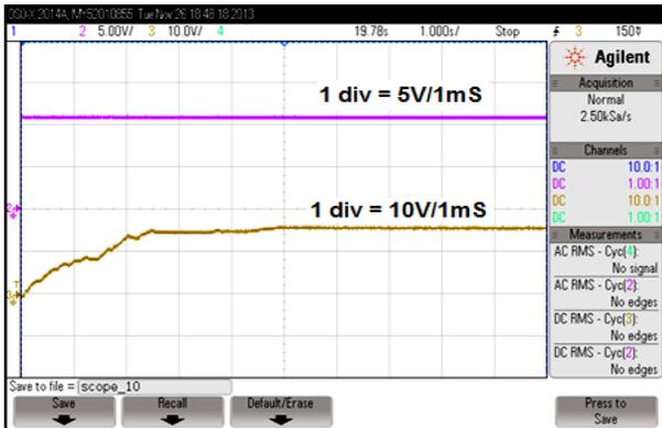
Fig.16 Output signal obtained for 12V input,  $V_{ref} = 16\text{ V}$
