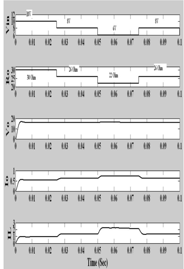
Fig.9. Output response of the boost converter along with discrete PID controller ( $V_s$  is the input voltage,  $R_o$  is the load resistance,  $V_o$  is the output voltage,  $I_o$  is the output current, and  $I_L$  is the inductor current)
