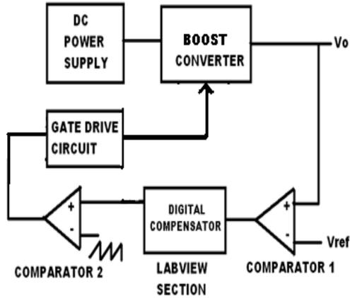
**Fig.1.** Block diagram for digitally controlled Boost converter
