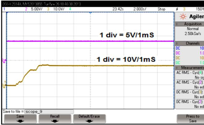
Fig.15 Output signal obtained for 8V input,  $V_{ref} = 16\text{ V}$
