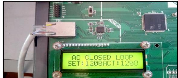
Fig. 14(c). Reference and actual speed display for closed loop.
