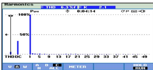
Fig. 15(e). Stator current THD at the load of 1.2 A on open-loop.
