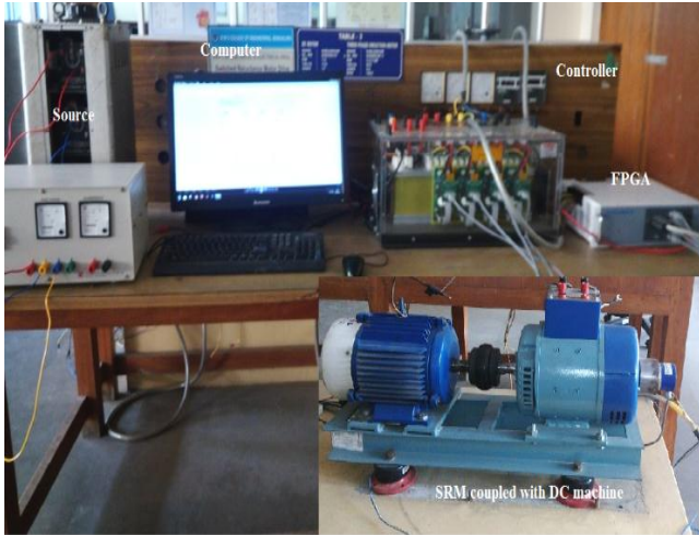
Fig. 12. Experimental Set-up for control of SRM.
