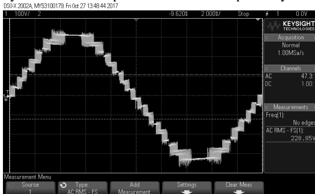
Fig. 15.a. Output voltage waveform of 15level MLI with single DC source and splitting capacitors
