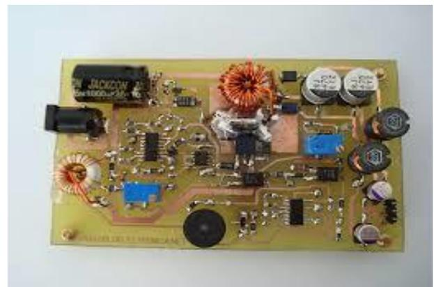
Fig. 8. Experimental model of ASM controller
